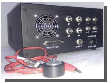
Nuline VECTRA CNC controller box is a bridge between CNC software and CNC machine. Vectra CNC is equipped with 3 Linear axis (X,Y and Z). Controller has the dedicated emergency stop push switch and supports safety limit switch by sensing the signals from limit switches from all the 3 axis. The controller comes with RPM knob to maintain the speed of spindle for different applications.
